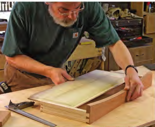
Sliding home. The drawer bottom slides past the drawer back and into grooves in the sides and front. Screws in elongated holes will hold the bottom to the back and allow the bottom to shrink or swell.
